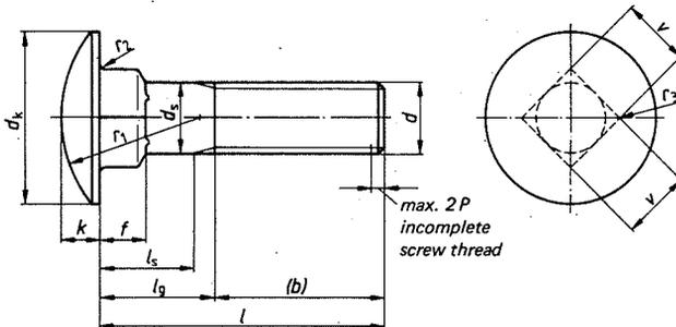
Designation of a mushroom head square neck bolt, with screw thread  $d = M 10$ , length  $l = 70$  mm and strength category 3.6 or 4.6 (at manufacturer's discretion):
